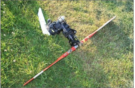
Figure 13: The tail rotor was found torn away from the tail boom
