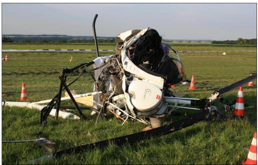
Figure 12: tail boom on the left - rotor blade in front showing no major bending
