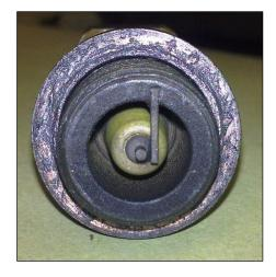
Figure 17: electrodes of one spark plug
