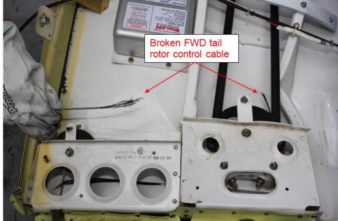
Figure 11: broken control cable
