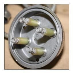
Figure 16: grease on the HT leads spring ends
