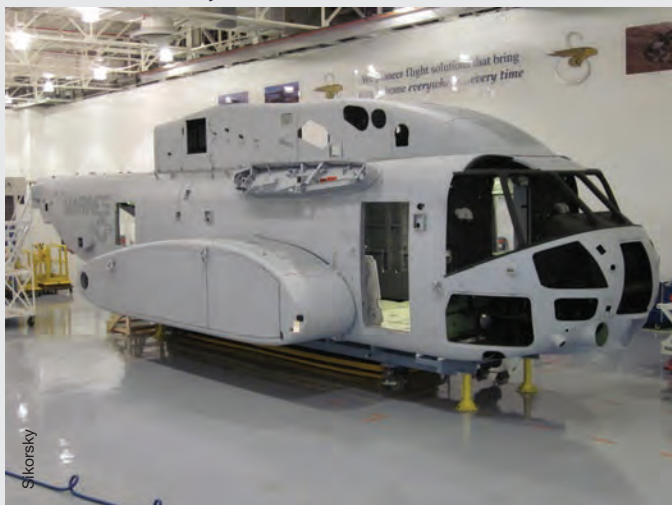
Final assembly of the first CH-53K is taking place at Sikorsky's new Florida Assembly and Flight Operations (FAFO) center in West Palm Beach.
