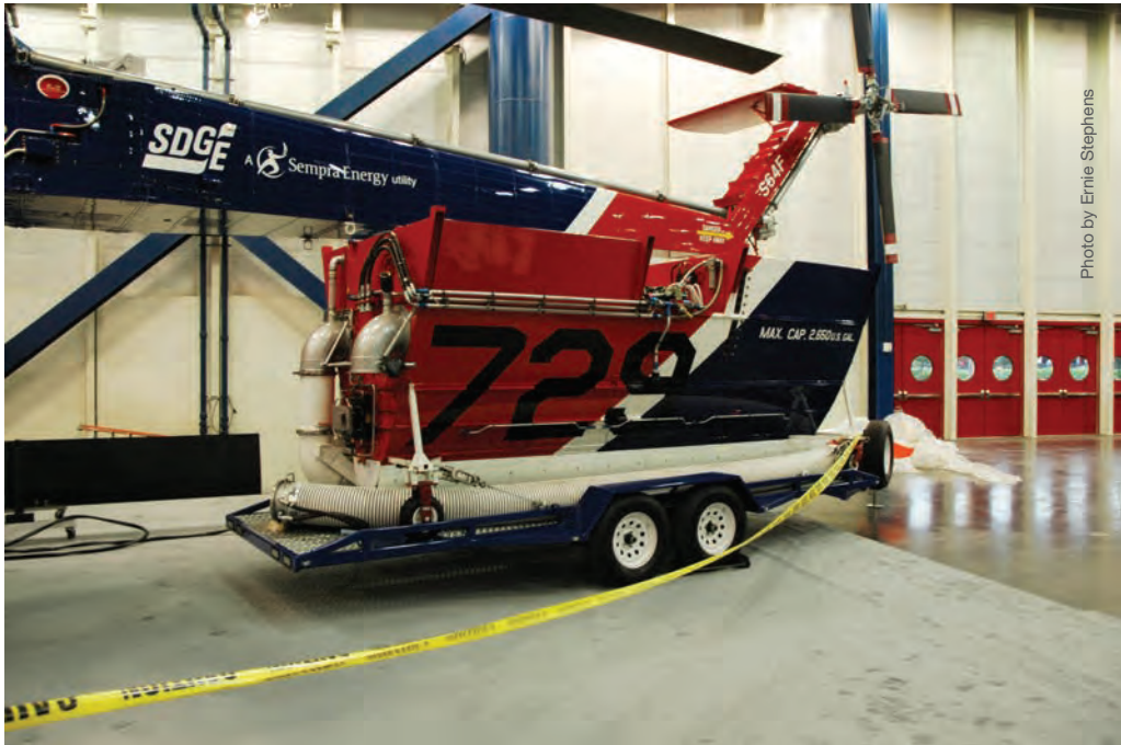
San Diego Gas & Electric's red, white and blue S64F Air Crane is primarily used for power grid construction and maintenance, but has a matching, detachable tank that can carry 2,650 gallons of water. It can draw its load from ground tankers, or through one of two snorkels lowered into a water source.
