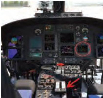
The X3's instrument panel varies little from its cousin the EC155. The primary differences are the test gear mounted atop of the glare shield, a special power management display (PMD) for the propellers (circled), and the thrust control lever (indicated by the arrow).
