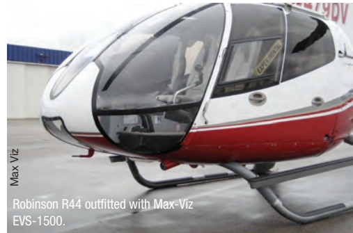
Robinson R44 outfitted with Max-Viz EVS-1500.
