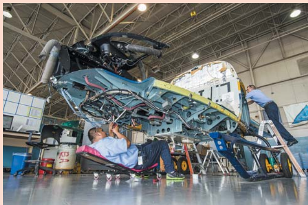
Above: Airbus Helicopters carry out 12 year inspections for US and Canadian operators of the EC120 and AS350 family at their Grand Prairie, Texas and Fort Erie, Ontario facilities. This is an EC120 under overhaul for the Albuquerque Police Department.
