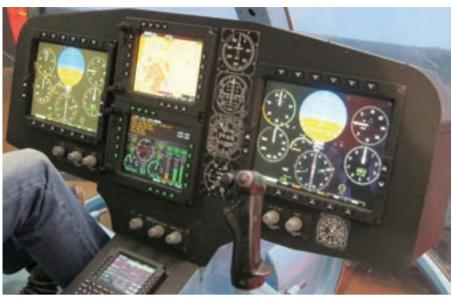
This view of a simulator shows the Ka-226's typical cockpit layout, with flat-panel displays plus analogue backup instruments. (Photo: author)
