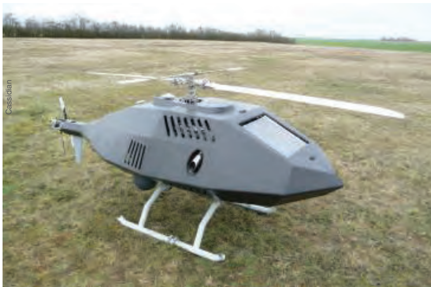
Tanan 300 vertical takeoff and landing tactical unmanned aerial system (VTOL Tactical UAS) from Cassidian.
