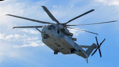
To conduct expeditionary heavy lift assault transport of armored vehicles, personnel and equipment to support distributed operations deep inland from a sea-based center of operations.
