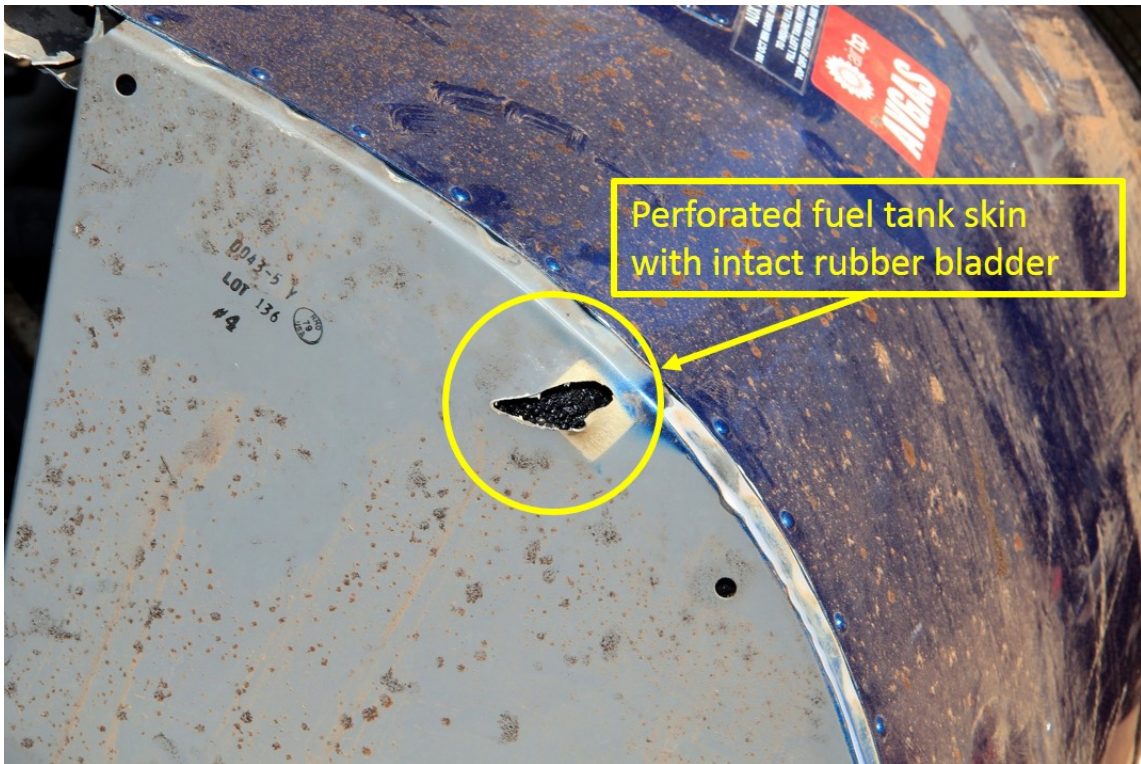
Figure 4: Perforated auxiliary fuel tank outer aluminium skin. Note the intact rubber bladder tank (circled in yellow)
