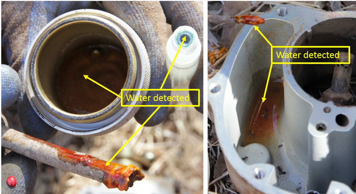
Figure 5: Gascolator (left) and carburettor (right) showing fuel contamination as indicated by the change in colour of the water detecting paste to red
