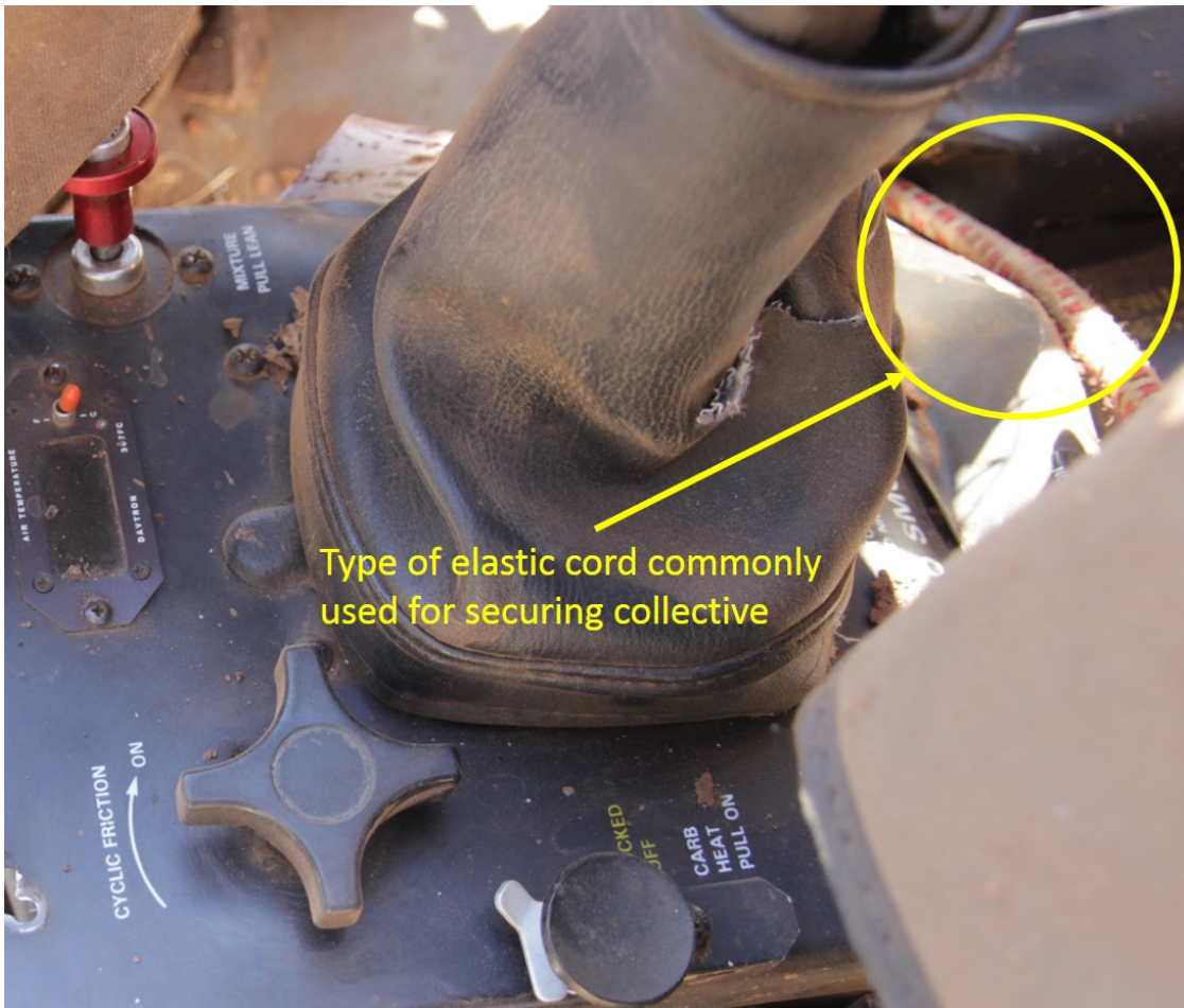
Figure 11: Elastic strap found positioned near the collective (such as reported used by some pilots to secure the collective lever)
