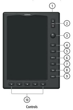
Press and hold to turn the unit on or off With the unit on, press to adjust the backlight and volume **RNG Key** Press to increase or decrease the viewing range of the map
