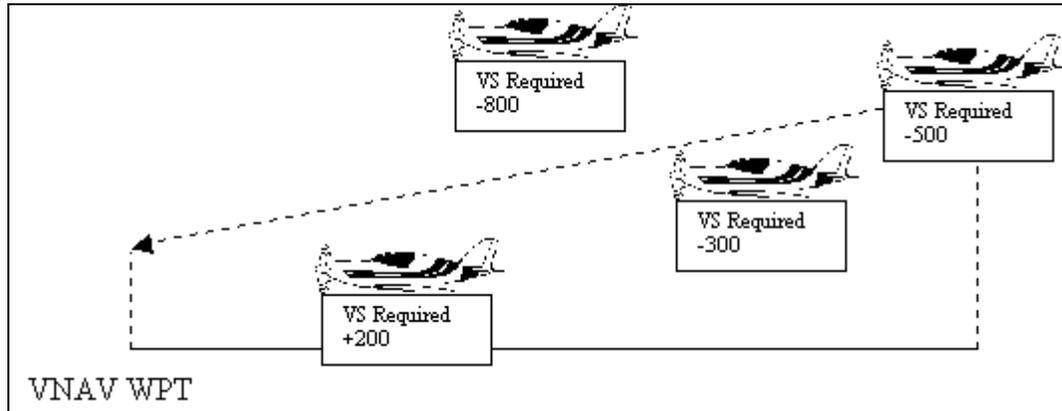
**Figure 9-8 VS to Target (not to a precise scale or value)**
