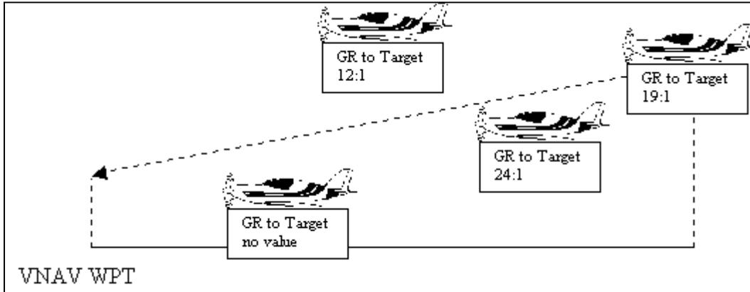
Figure 9-9 GS to Target (not to a precise scale or value)
