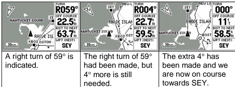
Figure 7-9 Navigating to a point using bearing information.
